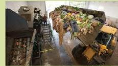
A bio-separator recovers the virtually odorless liquid material for use as natural cropland fertilizer, reducing the need for petroleum-based chemicals
