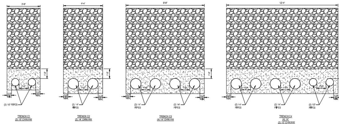
**HEATING/COOLING PIPE TRENCHES** (A1)
