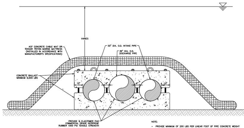
PROVIDE 1/4 ELASTOMER PAD - COMMERCIAL GRADE NEOPRENE RUBBER 1000 PSI TENSILE STRENGTH
